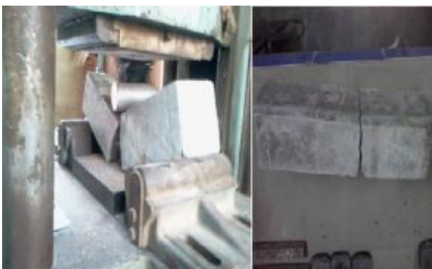
Fig.7: Flexure Strength Test
